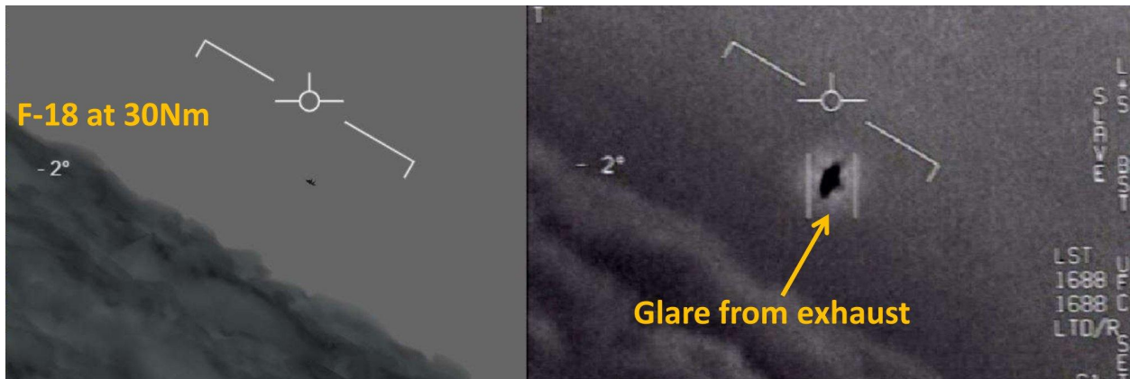
Figure A8. Comparison between the estimated size of an F/A-18F at 30 nautical miles (left, in the 0.35° NAR2 FOV for the ATFLIR, https://www.metabunk.org/sitrec ) and the end section of the Gimbal video (right). The NAR2 FOV is a digital zoom (x2) of the narrow optical zoom NAR1, FOV 0.7°. One pixel of the NAR1 FOV corresponds to ~4-5 ft at 30 Nm, following the formula: size(ft) = 2 * \tan(FOV/2) * dist(Nm) * 6076.12(Nm \text{ to } ft) / 480(\# \text{ pixels on width}) . At that distance, the heat source (F/A-18F exhaust nozzles) has an equivalent size of just a few pixels of the infrared camera.
