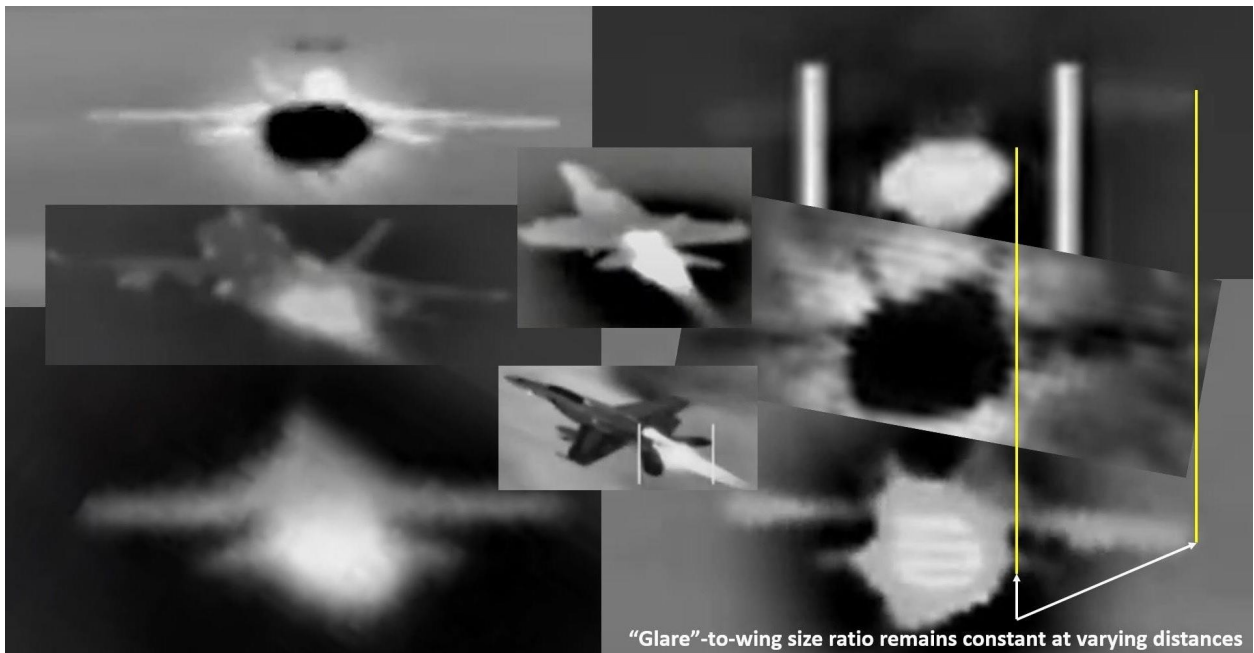
Figure A10. Publicly available AN/ASQ-228 ATFLIR imagery of F/A-18 jet engine exhaust. In the available ATFLIR footage, exhaust viewed approximately tail-on never obscures the entire aircraft by several factors, as required by the "distant jet" theory (Figure A8).
